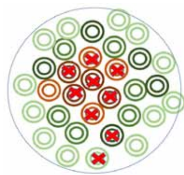
Illustration of bamboo clump showing bamboo culms to cut to create a horseshoe opening
